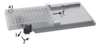
4 Close the catch and make sure that the microplate is properly seated on the rack tray.
