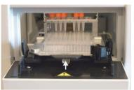
2 Lift the rack tray slightly and take it out of the instrument.
