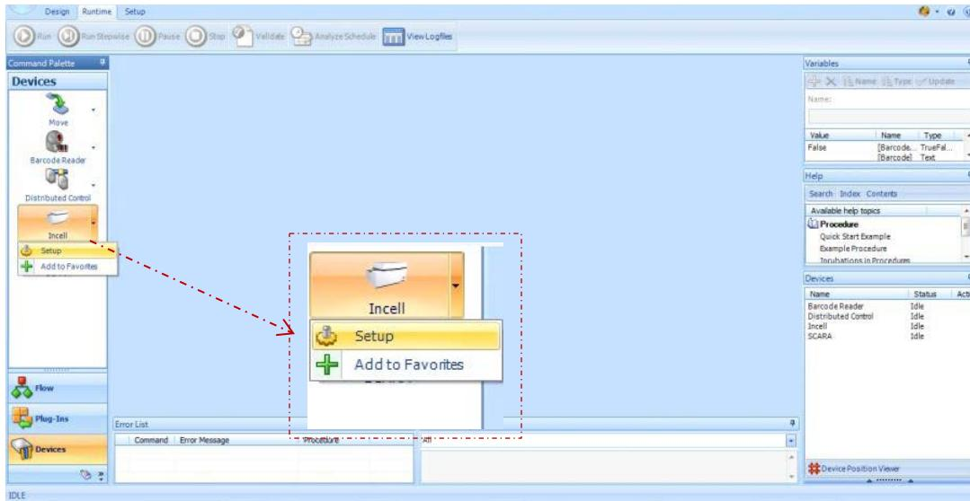
3. On the **GE InCell Setup** dialog, increase the **Read Timeout** interval to 1000 minutes, or longer if using a driver version above 1.0.3.20.
