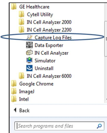
The Capture tool helps simplify the process of retrieving log files from remote sites. Reducing the number of steps involved with gathering log files streamlines the process of diagnosing and repairing acquisition-related issues. To use the Capture tool, add a brief comment about the situation, select the appropriate files, and then select **Create ZIP**. By default, log files are stored on the user's desktop.
