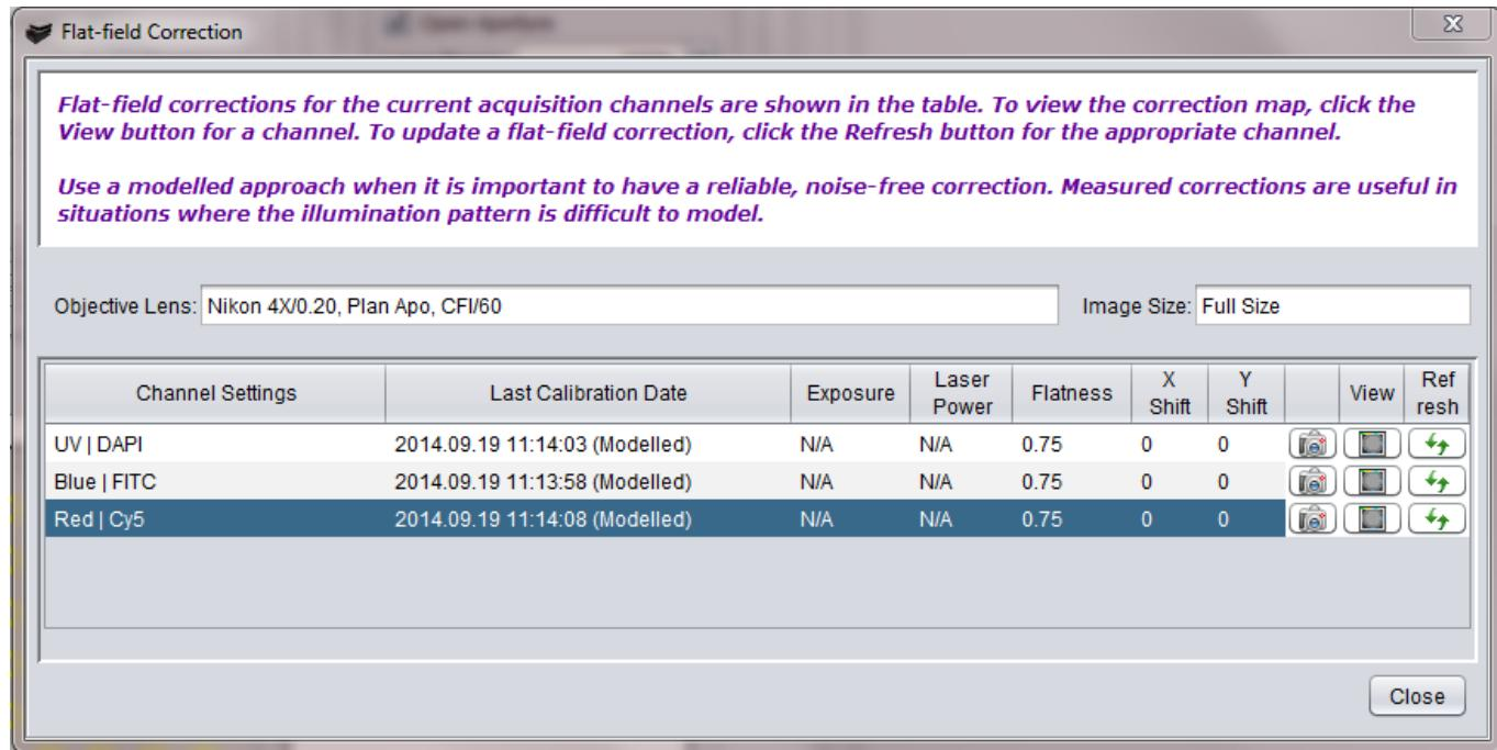
Modelled FFC maps are good for situations where it is difficult to measure an accurate flat-field calibration. Modelled FFC maps do not contain noise, which means that the calibration process will not affect image quality.
