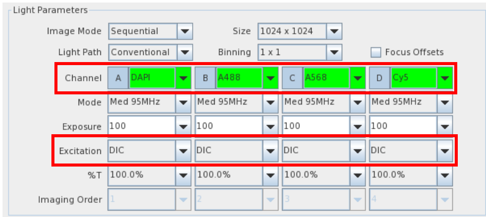
Figure 6. Activate All Cameras and Set Excitation to "DIC"
