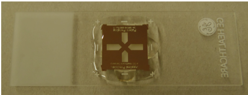
Figure 3. Image Alignment Slide, Target Faces Toward Objective
